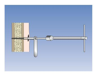
Remove the drill bit and drill guide, keeping pressure on the handle of the screw guide.
