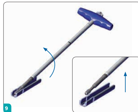
9 Main lag screw connection
