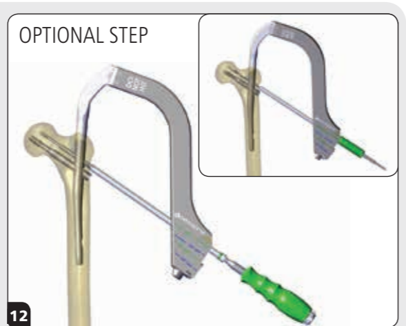
12 OPTIONAL STEP Insertion of the supplementary lag screw
